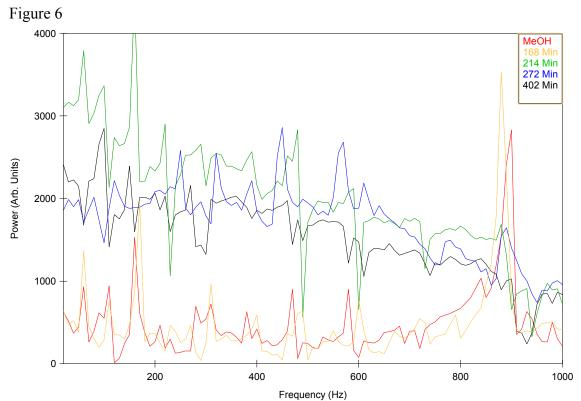
This is a graph of 4 different data sets taken from the 98% sample at various point in time, along with the control. At 168 minutes, the gelation had finished, but the sample was not yet vibrating (this occurred at 184 minutes).
