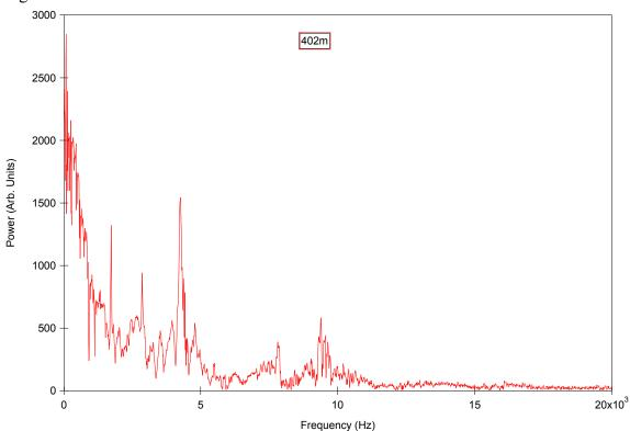
This is the same 98% gel shown above 402 minutes after preparation. The vibrations in the liquid were obviously discernable when the sample was felt, and had been since 184 minutes had passed.
