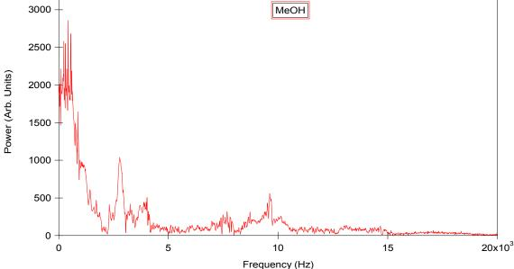
A Glass container identical to the ones used for the alcogels was filled with methanol and excited. The same clamping and transducer conditions were kept. This sample was taken just prior to the 98% gel was prepared.
