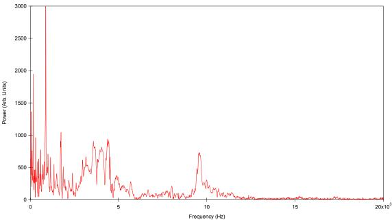
This is a 98% gel data set taken 168 minutes after the sample was prepared. This set was taken once the liquid appeared to have completely solidified when visually examined, but vibrations could not be sensed when felt. It is in an identical container and uses the same clamping and transducer conditions as used in the control.
